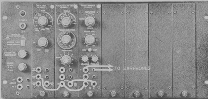
Figure 2-12. Type 1395 Series modules connected to test musical tones.
