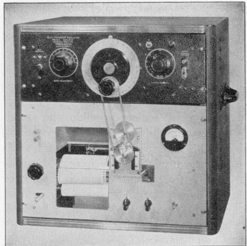
Figure 2. View of the Model FR-1 Graphic Recorder with the Type 913-C Beat-Frequency Oscillator.
