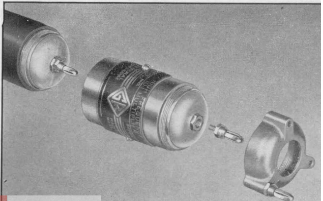
Figure 1. Exploded view of probe, multiplier, and cap.
