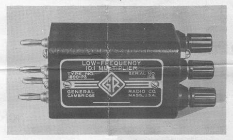
This multiplier extends the range of the Type 1800-A Vacuum-Tube Voltmeter to 1500 volts for both d-c and low-frequency a-c measurements. The multiplier plugs into the binding posts on the voltmeter panel. For d-c measurements a fixed resistance voltage divider is used giving a 10:1 reduction in the voltage applied to the voltmeter. For a-c use the multiplier consists of a capacitance-resistance voltage divider.
