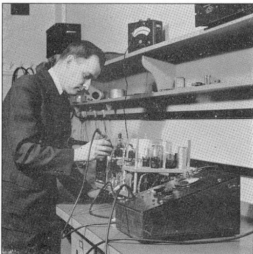
FIGURE 6. A. G. Bousquet of the High-Frequency Group, who has designed a number of General Radio's signal generators, vacuum-tube voltmeters and power supplies, is shown here testing a preliminary model of a standard-signal generator.
