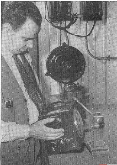
FIGURE 1. Mr. Frank Wilkins of the Barbour-Stockwell Company reading the relative positions of the drum dials by means of the Strobotac.
