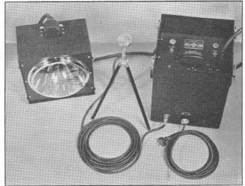
FIGURE 5. View of the Microflash Unit, consisting of light source, power supply, microphone, and connecting cables.
