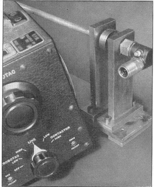
FIGURE 2. Close-up of the torque meter. The two drum dials, one carrying an index, the other a scale, are shown between the two vertical supports.
