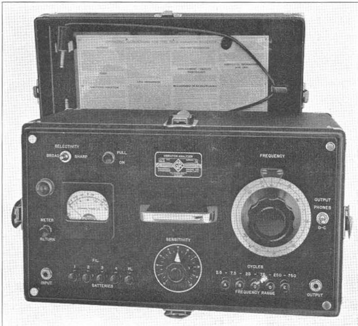
FIGURE 1. Panel view of the TYPE 762-B Vibration Analyzer.
