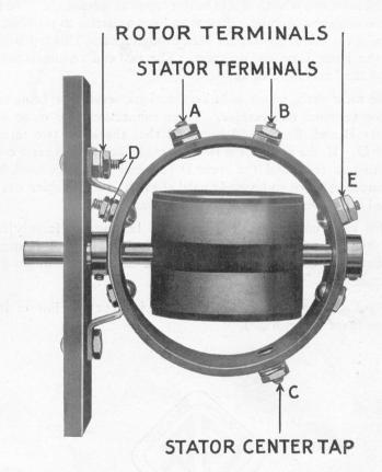
The type 268 Vario Coupler is designed particularly for the wavelength ranges of broadcast reception. The circuit should be so arranged that this band of wavelengths (200-600 meters) may readily be covered. Because of the large variety of circuits and of the varying conditions under which this vario coupler may be used it is not possible to recommend any one capacity of condenser to be used. Where the primary
