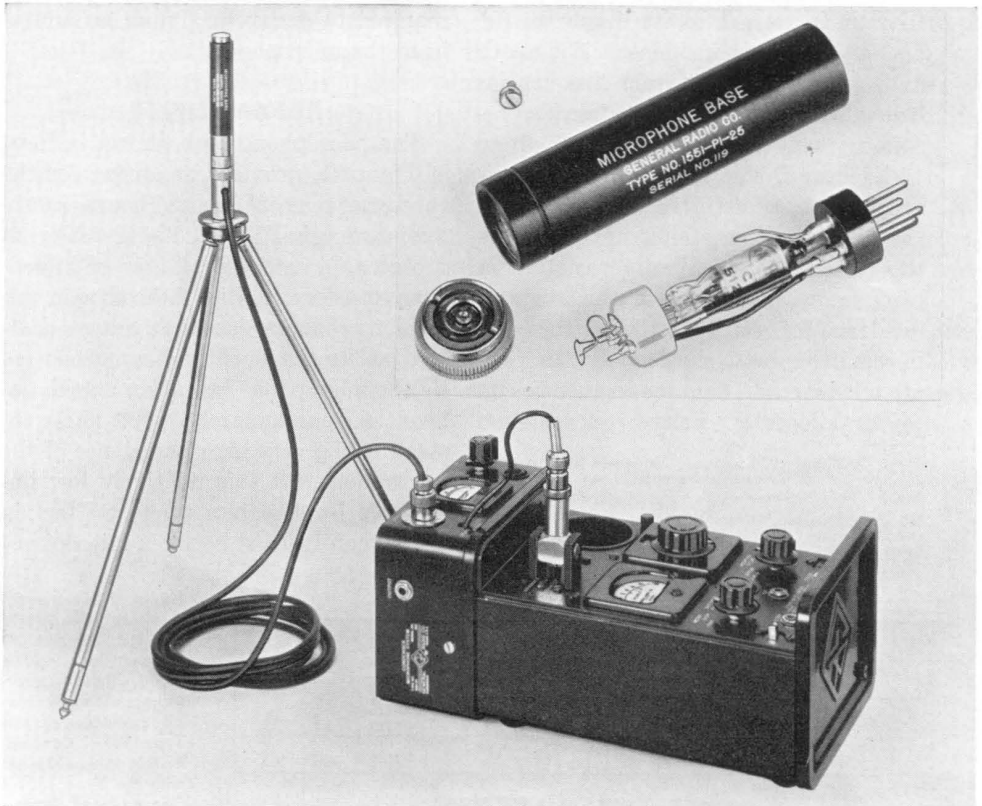
Figure 1. View of the Type 1551-A Condenser Microphone System attached to the Type 1551-A Sound-Level Meter. Inset shows microphone, microphone base, and preamplifier.
