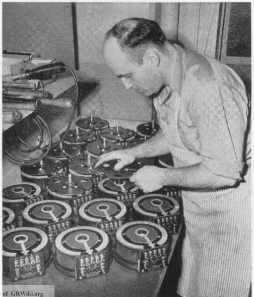
The Duratrak process, which follows baking, coats the brush track with the silver surface shown on these partially assembled units.
