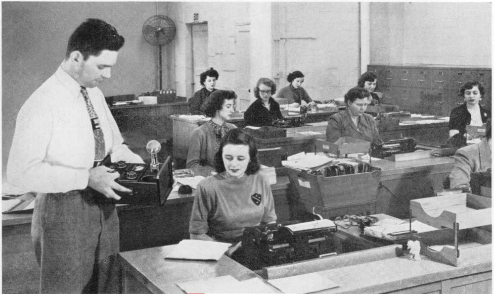
Figure 5. Determining noise level and speech-interference level in a business office with the Type 1551-A Sound-Level Meter.
