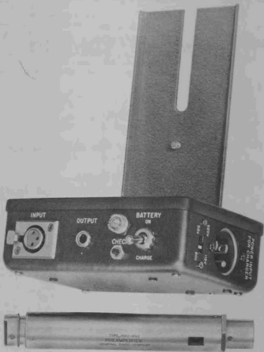
Figure 1-1. Type 1560-P40 Preamplifier with Type 1560-4100 Power Supply and mounting bracket.
