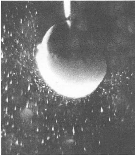
Figure 2. Icing of a 2-cm steel ball in an air stream (temperature -25^{\circ}\text{C} ); diameter of the arriving ice particles or subcooled water droplets 50\text{-}100\ \mu . Observe the "boundary layer" of the rebounding particles. For this photograph, a slot illumination (slot opening 2 mm) was used, necessitating a camera opening to f/1.6 . The visible diffraction pattern (rains) results from reproduction of cloud droplets passing the steel ball at a distance of more than 2 cm in the direction of the camera.
