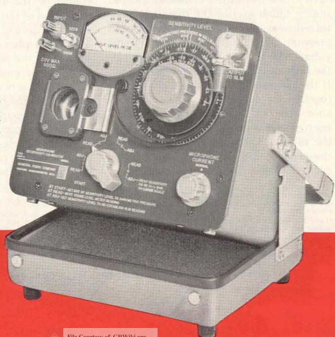
Figure 1. The Type 1559-A Microphone Reciprocity Calibrator is supplied in a Flip-Tilt case for convenient bench use. A relay-rack model is also available.
