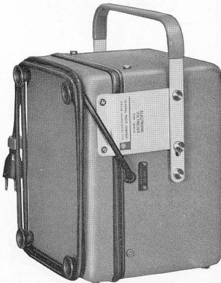
Figure 11. The Type 1806-A Electronic Voltmeter with cover closed and the power cord around the rubber feet for storage or transporting.
