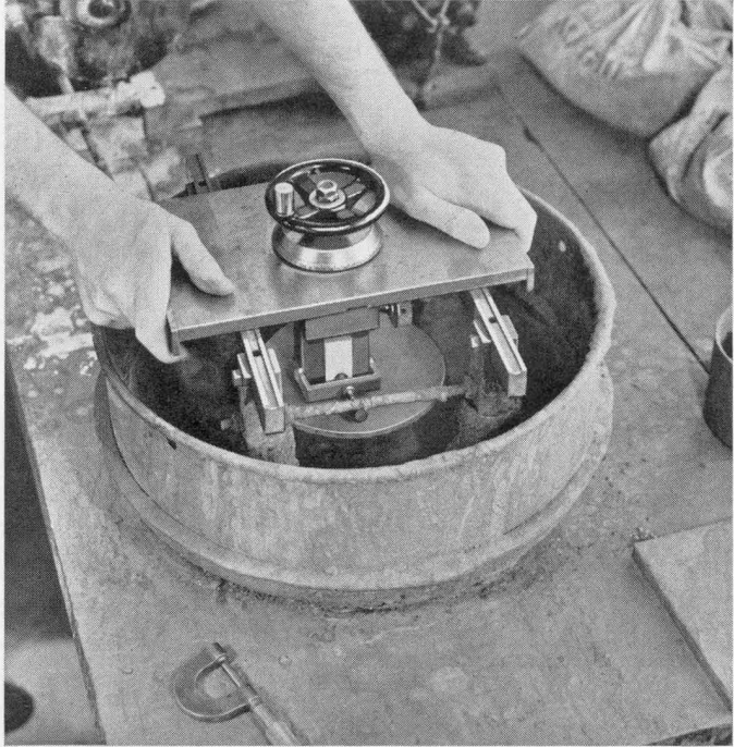
FIGURE 4. One of the grinding operations in the production of General Radio quartz plates. The edge of the plate is held against a rotating disk, and the calibrated head shows the amount ground from the edge
