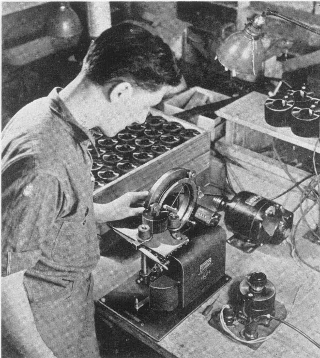
TYPE 200-B Variacs are wound on the machine shown above
