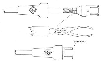
priate die and squeeze the handles together until the ratchet lock releases.
