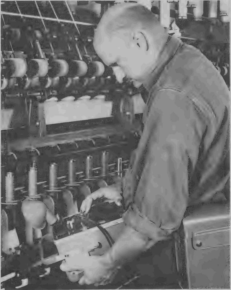
Figure 1-4. The Type 1538, powered by the Type 1538-P3 Battery pack, offers a precise bright stroboscope capability in a completely portable format, a unique advantage in use with large machine complexes such as found in textile and printing industries. The battery pack can power the strobe for up to 8 hours of intermittent use.
