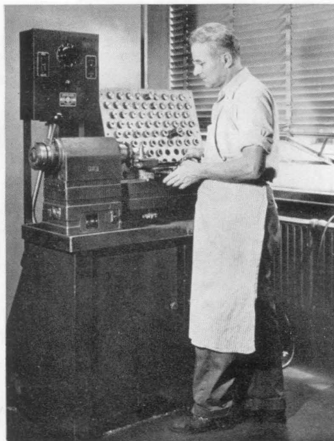
Figure 2. Typical installations of the \frac{3}{4} -hp Variac Speed Control, (left) on a lathe, and (right) on a toroidal winder.
