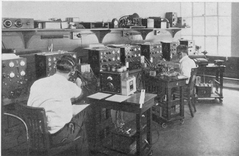
Calibrating a group of special self-checking heterodyne wavemeters designed and built by General Radio for the United States Coast Guard
