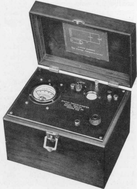
TYPE 532 Station Frequency Meter
