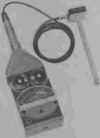
Figure 6. The sound-level meter fitted with the Type 1560-P96 Adaptor and the Type 1560-P52 Vibration Pickup.
