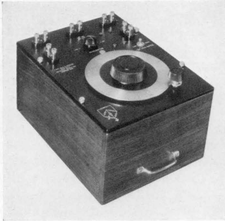
FIGURE 2. TYPE 625-A Bridge
