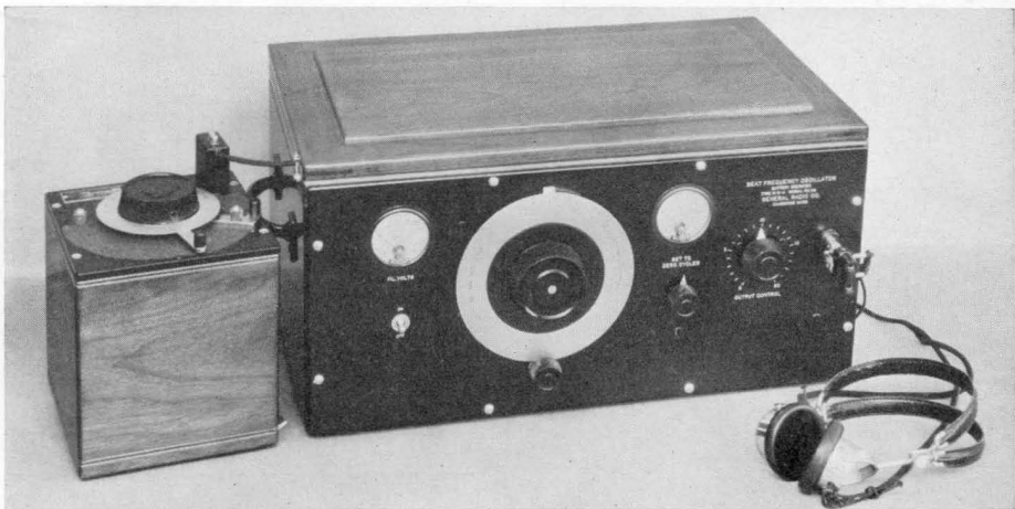
Any pitch between 5 and 10,000 vibrations per second is obtainable from the TYPE 613-B Beat-Frequency Oscillator. Incremental variations on either side of a given frequency are obtained by means of the condenser at the left
