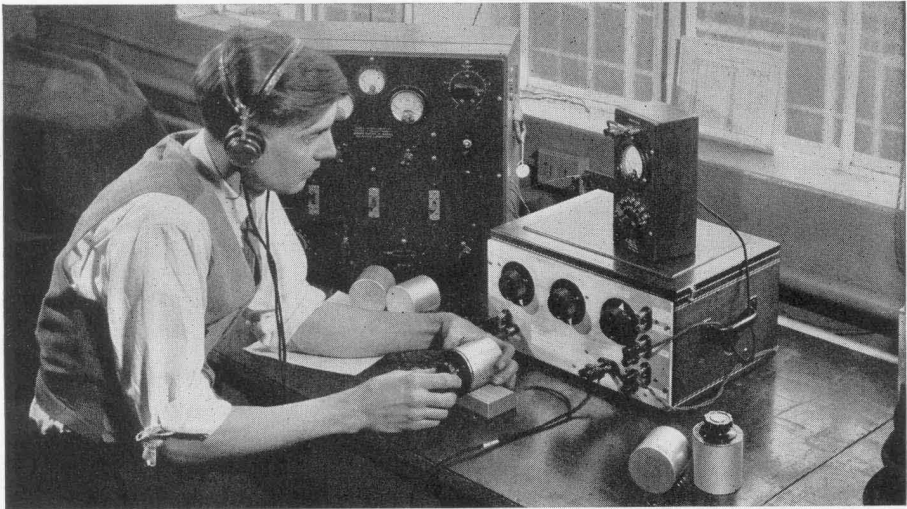
FIGURE 5. Inspecting TYPE 653 Volume Controls for noise. Every General Radio volume control is individually tested for noise, attenuation, and impedance, as well as the usual mechanical inspection
