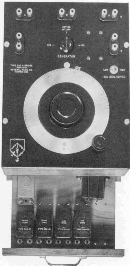
FIGURE 1. The skeleton-type bridge with the drawer pulled out to show the method of storing standard resistors and condensers when not in use
