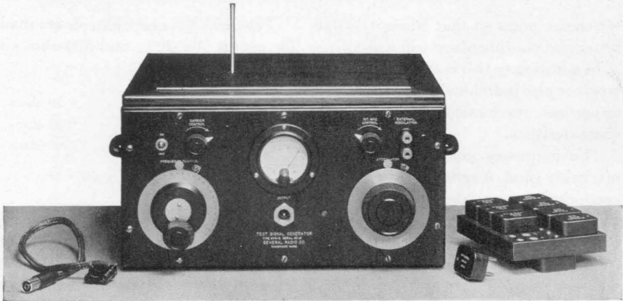
FIGURE 1. A TYPE 604-B Test-Signal Generator showing the smallest of the three rod-type antennas. Voltage can also be delivered to the receiver under test by means of the cable, the jack for which is on the panel. The coil-mounting rack and the 13 coils supplied with the instrument can be stored in a compartment inside the cabinet
