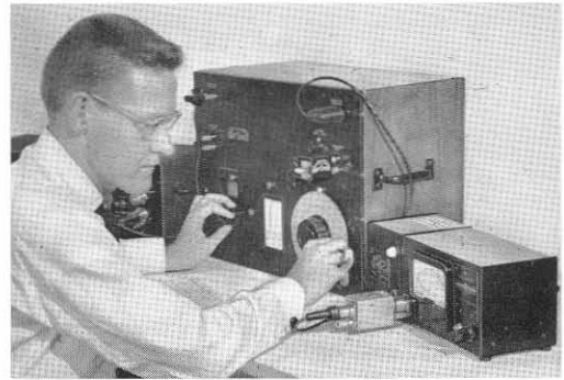
Equipment for 1-mc capacitance measurements. The generator is the Type 1330-A Bridge Oscillator, the bridge the Type 716-CS1 Capacitance Bridge. The null detector (Type 1212-A) is shown at the right. The filter shown is the experimental model; the Type 1212-P2 plugs into the detector in the same way.
