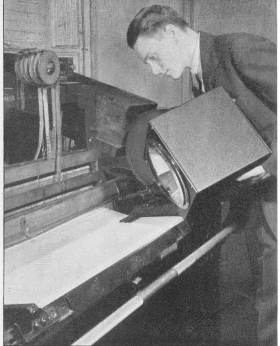
FIGURE 10. Photo courtesy Hoosac Mills, New Bedford, Mass. Experimental loom operating at 180 picks per minute. Long rod in foreground was geared to a make-break contactor so that the exact phase of flash could be set by hand.
