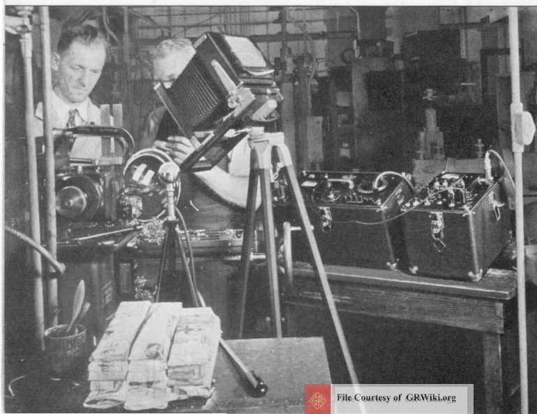
FIGURE 12. Set-up for taking photographs with TYPE 759-A Sound-Level Meter, TYPE 760-A Sound Analyzer, TYPE 631-B Strobotac, and TYPE 648-A Strobolux. The camera shutter is opened and closed by hand; the Strobolux is flashed at any particular frequency of sound selected by the Sound Analyzer.
