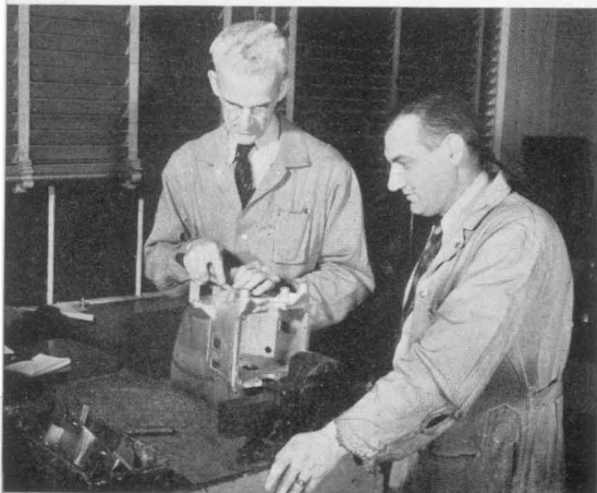
Measuring a condenser frame casting preparatory to making a drilling jig. (Left to right) E. S. Page (who is also president of the GR Credit Union) and G. G. Oberbeck, foreman of the tool and screw machine department.
