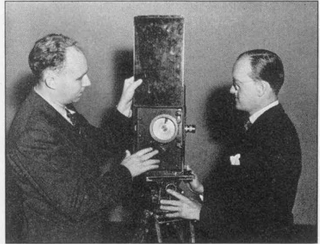
Dr. Edgerton explains the operation of the high-speed camera to Pete Smith, Commentator of "Quicker'n a Wink." This camera will take pictures at the rate of 1500 frames per second.
