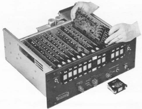
Figure 10. Plug-in etched boards are easily removed for service or replacement.
