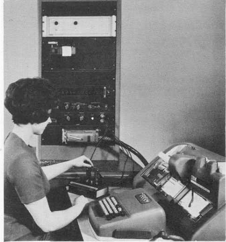
Fig. 9. IBM Model Printing Summary Punch operating from output of automatic bridge. Capacitance values are automatically punched; operator adds serial numbers. Also in relay rack are data printer and (top) intercoupler required for parallel-to-serial conversion.
