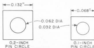
Figure 4. Cross section of internal coaxial leads.
