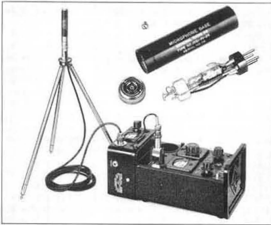
View of the condenser microphone system and sound-level meter, showing how power-supply assembly attaches to sound-level meter cabinet. Inset shows microphone, preamplifier and base, disassembled.
