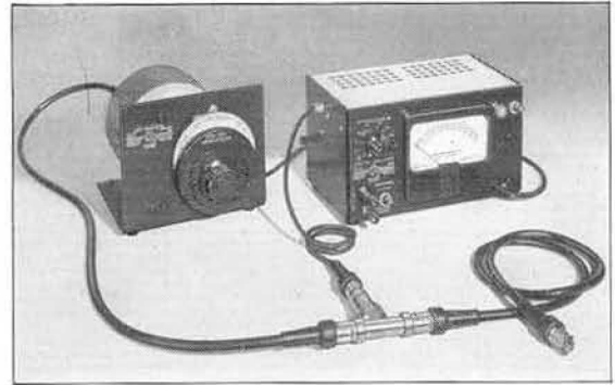
The TYPE 1216-A I-F Amplifier set up for use as a high-frequency detector, using a TYPE 1209-A Unit Oscillator as a heterodyning oscillator and a TYPE 874-MR Mixer-Rectifier.
