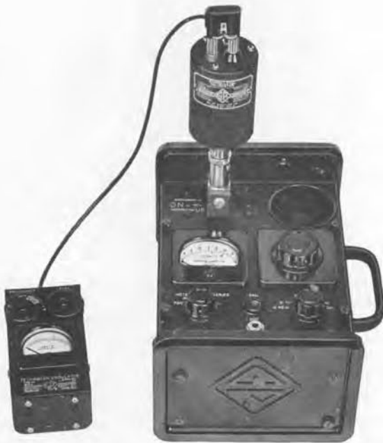
Calibrator fits over microphone as shown above. At left is the TYPE 1307-A Transistor Oscillator.
