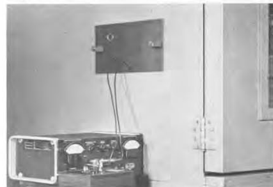
The built-in guard circuit permits the use of long leads from Comparator to sample inside conditioning chamber, as shown above.
