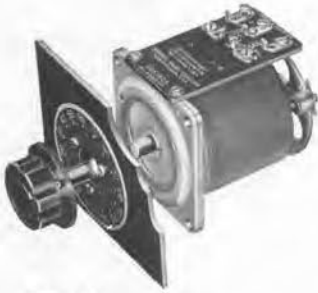
Type W2 Uncased Model. Mounting Base: 3\frac{1}{4} inches square. Depth Behind Panel: 3\frac{15}{16} inches. Four Mounting Holes on 2\frac{3}{4} -inch square. Max. Panel: \frac{3}{8} inch.
