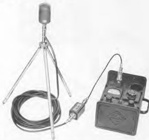
(B) Microphone and transformer plug into the sound-level meter as shown above.
