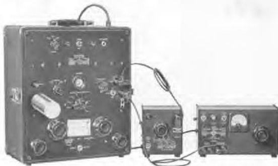
TYPE 1611-AS2 Capacitance Test Bridge used with the TYPE 1214-AS2 Oscillator to measure an electrolytic capacitor. The TYPE 1204-B Unit Variable Power Supply on the right supplies the d-c polarizing voltage.
