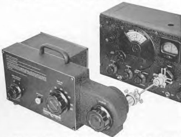
The sweep drive attached to the tuning knob of a short-wave receiver.
