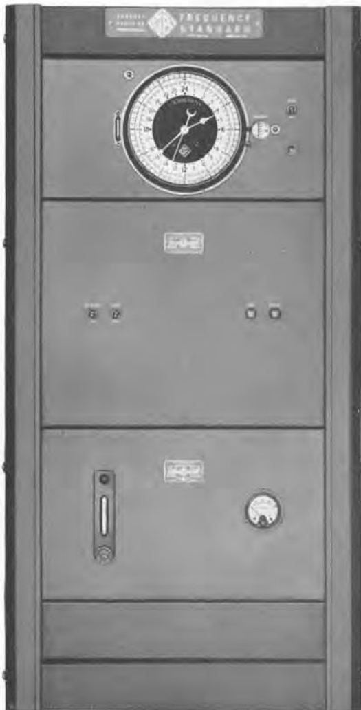
Close-up view of the TYPE 1100-AP Primary Frequency Standard. Lower part of the floor-type relay rack is not shown. The complete rack is similar to that shown in the photograph on page 77.
