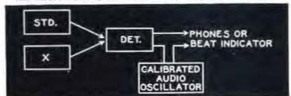
FIGURE 5. Functional diagram showing the operation of the direct-beating method of frequency measurement.
