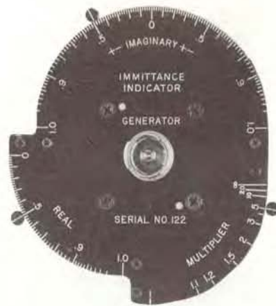
Dial calibrations of Transfer-Function Indicator (left) and Immittance Indicator (right).
