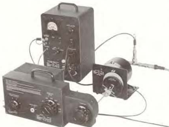
TYPE 1750-A Sweep Drive and the TYPE 1263-A Amplitude Regulating Power Supply set up to sweep a TYPE 1209-B Unit Oscillator, thus providing a constant sweep output over a frequency span of 250 Mc to 920 Mc. The equipment shown here is listed above, with the exception of the oscillator.
