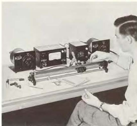
TYPE DNT Detector used with the TYPE 874-LM Dielectric Measuring Line to measure the dielectric constant and dissipation factor of solid-dielectric materials.
