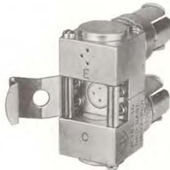
Transistor mounts available for making reproducible measurements on transistors having JETEC-30 base arrangement. TYPE 1607-P101 grounds the base lead; TYPE 1607-P102 grounds the emitter lead and both have removable, oscillation-damping resistor. Spring holds transistor firmly in place and grounds case.
