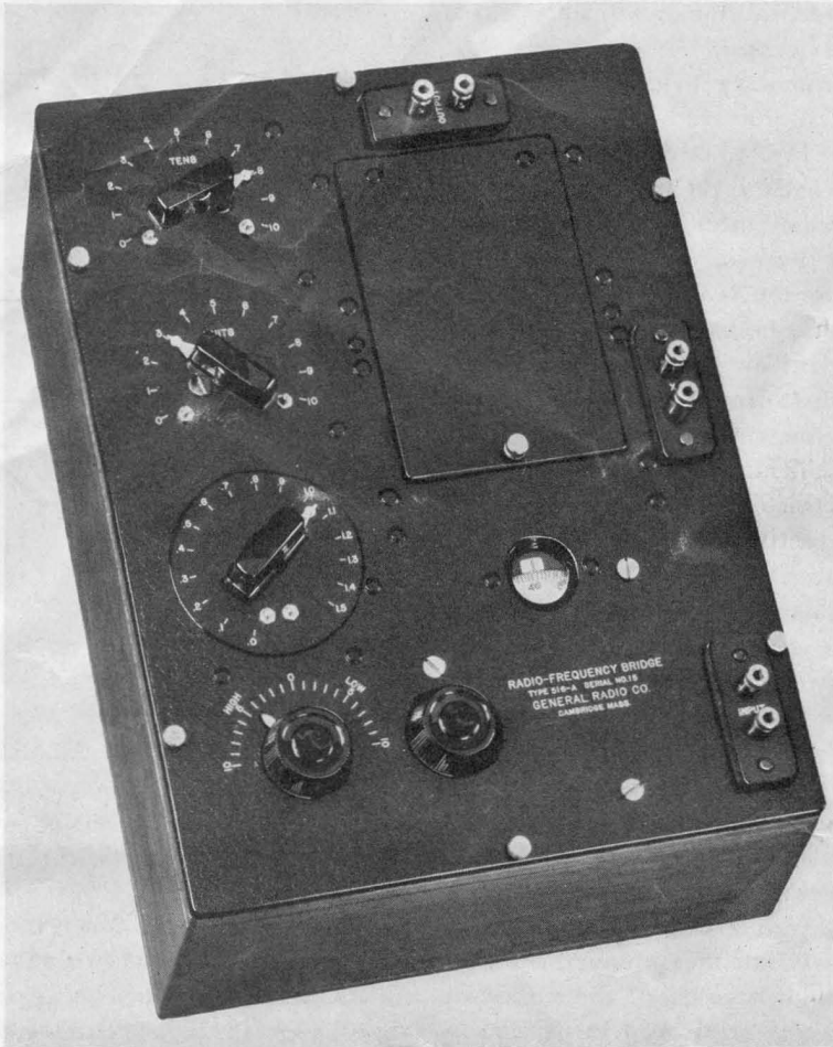
FIGURE 2. The new TYPE 516-A Radio-Frequency Bridge, an experimental instrument for the determination of reactance and resistance at high frequencies. Its use is recommended for laboratories having a considerable experience with other methods for measuring impedance
