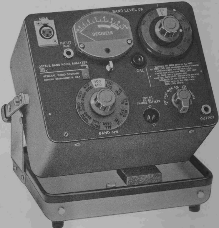
Figure 1-1. Views of the Type 1558-A Octave Band Noise Analyzer. (Above, left) in relay-rack adaptor; (above, right) case closed; (right) with microphone attached; (below) panel view.
