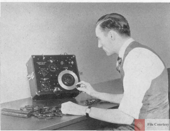
FIGURE 4. The capacitance test bridge set up for the rapid testing of mica condensers.
