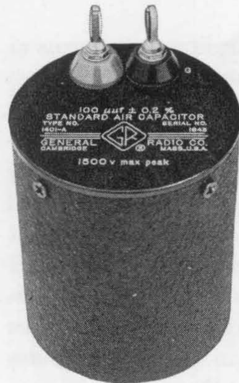
Figure 3. Type 1401 Fixed Air Capacitor as now supplied.
