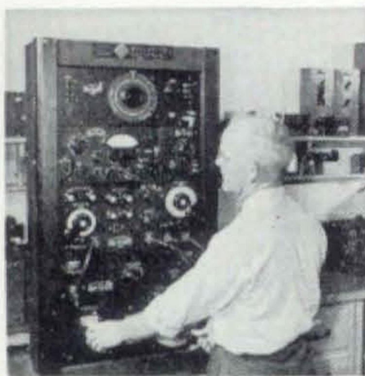
This scene in the General Radio Standards Laboratory shows the Type 1610-A Capacitance Measuring Assembly in use for the measurement of 3-terminal capacitors.
