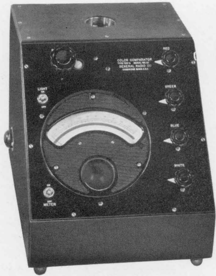
FIGURE 1. TYPE 725-A Color Comparator. Color intensity is indicated as a meter reading. Filters are shifted by means of the knob at the upper left. The pilot lamp indicates which filter is in position
