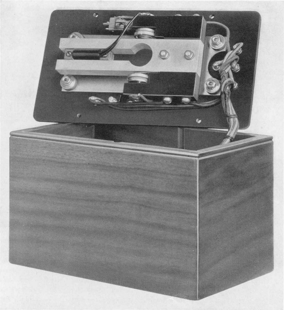
FIGURE 2. Internal view of 400-cycle oscillator, showing fork and method of mounting
