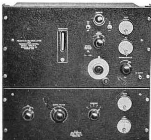
TYPE 592 and TYPE 575-AR assembled on a frame for convenience in making laboratory measurements
