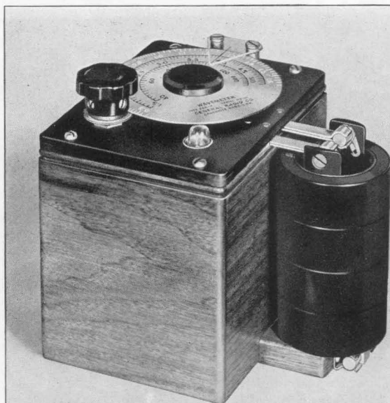
FIGURE 1. View of the TYPE 566-A Wavemeter showing how coils are stored when not in use.
