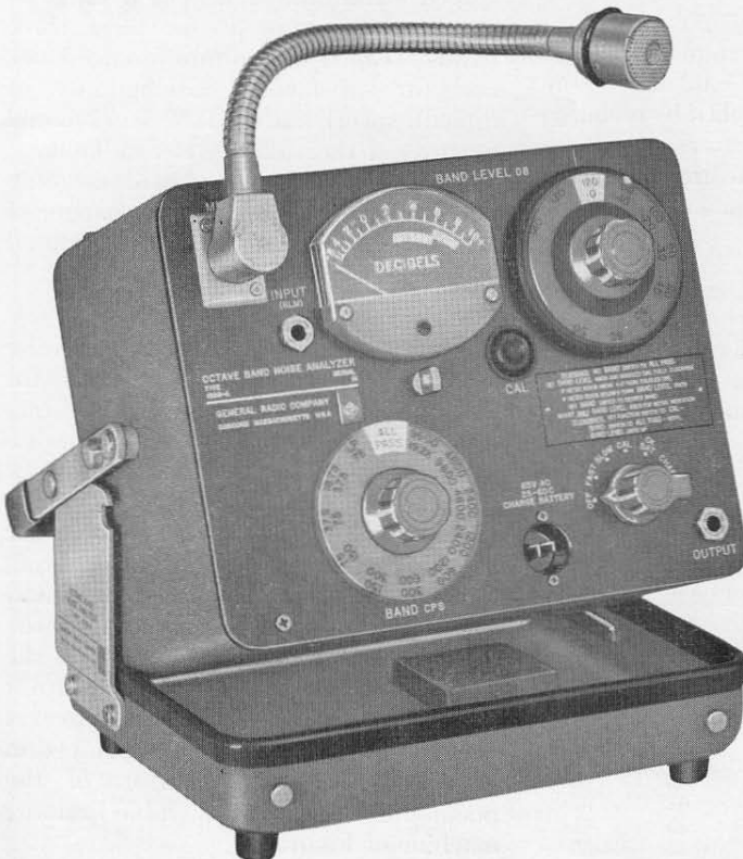
Figure 1. View of the Type 1558-A Octave-Band Noise Analyzer with the Type 1560-P4 PZT Microphone Assembly.
