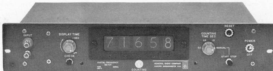
Figure 1. The Type 1150-A Digital Frequency Meter. Encased in General Radio's multi-purpose cabinet, 4 the instrument is readily mounted in a rack or adapted to table-top use with end frames. The panel is 3½ inches high. The controls and fittings are simple and clearly marked. Frequencies between 10 cps and 220 kc can be counted over preselected time intervals from 0.1 to 10 seconds. Display times can be continuously adjusted from 0.5 to 5 seconds and ∞.
