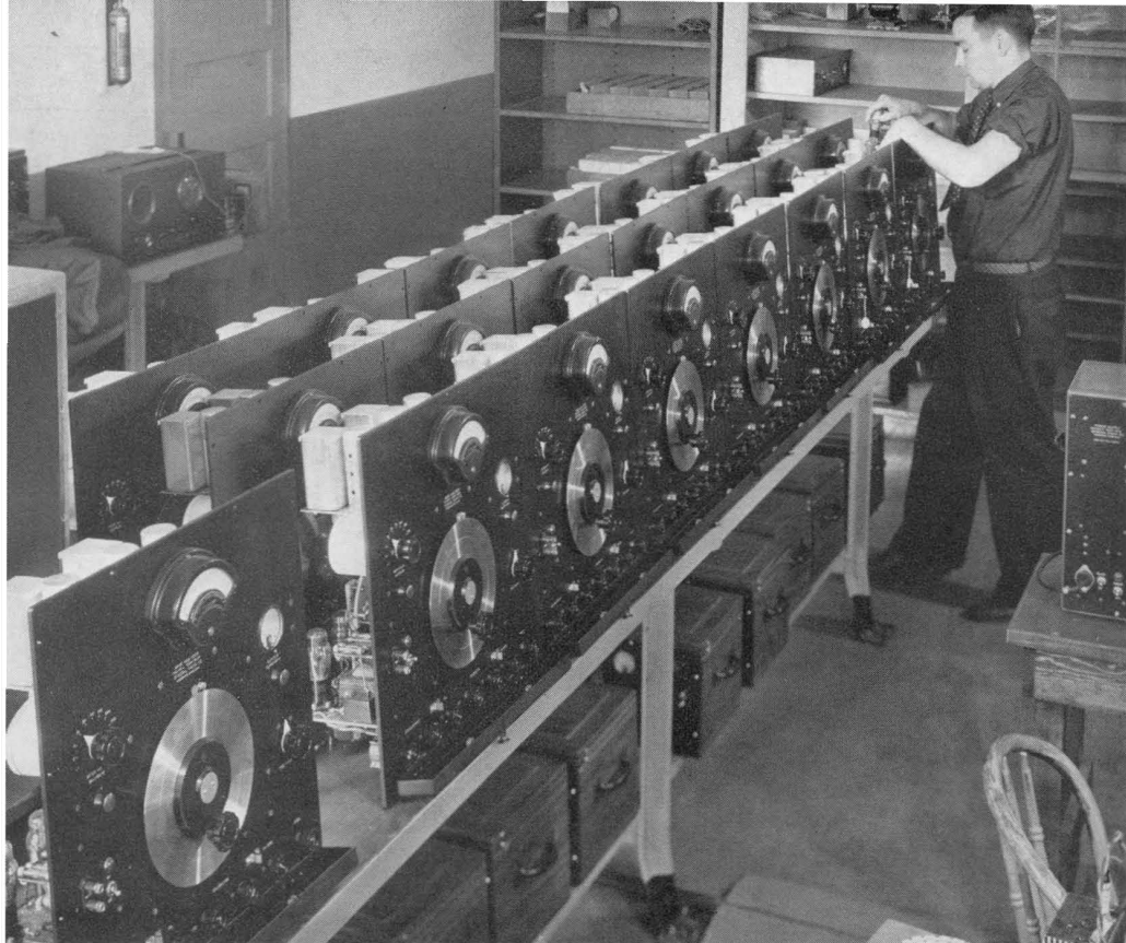
A group of TYPE 636-A Wave Analyzers under test in our calibration laboratory
