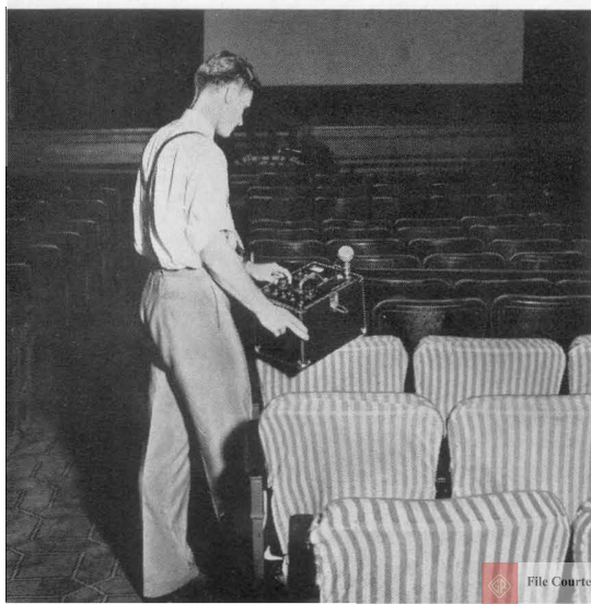
FIGURE 3. Measuring the acoustical properties of a motion picture theater with the sound-level meter
