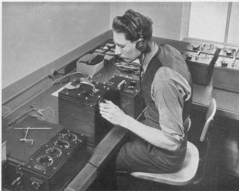
FIGURE 8. Calibrating a TYPE 722-F Precision Condenser
