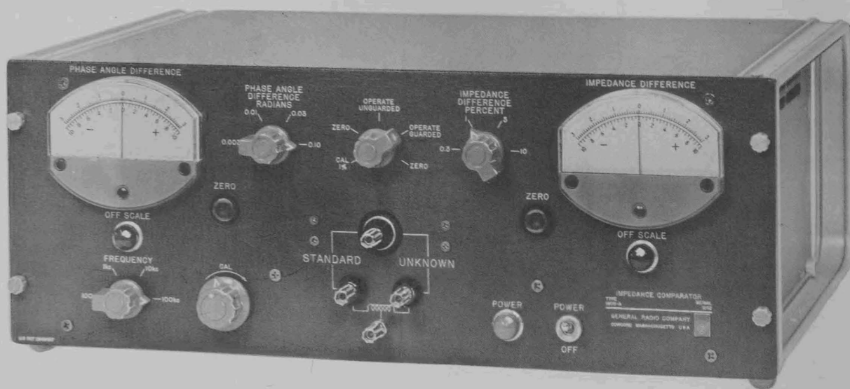
Figure 1. Panel View, Type 1605-A Impedance Comparator.
