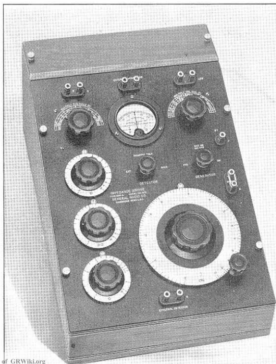
FIGURE 1. View of the TYPE 650-A Impedance Bridge with battery compartment at the rear.
