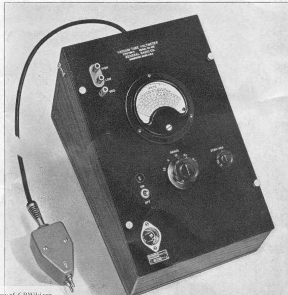
FIGURE 1. Panel view of the TYPE 726-A Vacuum-Tube Voltmeter, showing the probe in which the diode is housed.
