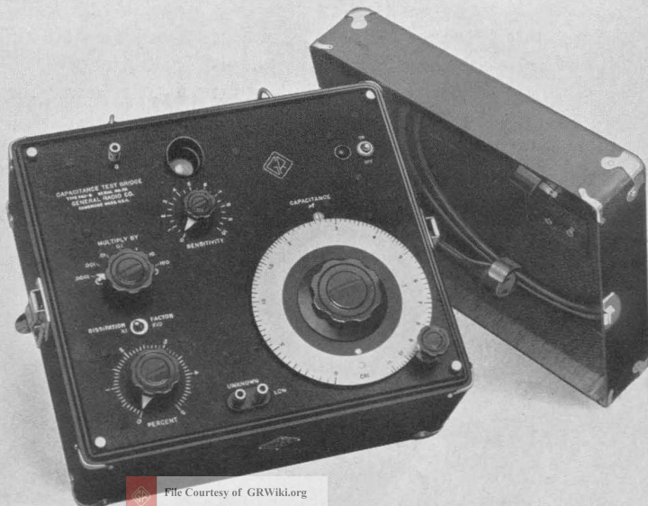
FIGURE 1. Panel view of the TYPE 740-B Capacitance Test Bridge with cover removed
