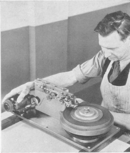
The self-indexing engraving machine which rules the scales on TYPE 704 and TYPE 706 Precision Dials
