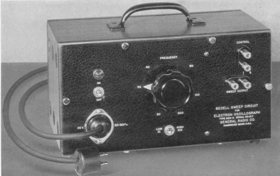
FIGURE 1. This new instrument supplies a controlled linear sweep for the General Radio TYPE 635 Electron Oscillograph
