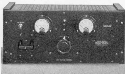
TYPE 673-A Power Supply. Practically any voltage from zero up to the rated maximum can be obtained from the high-voltage supply circuit of this unit
