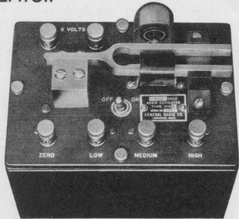
The 400-cycle TYPE 213-B Audio Oscillator whose waveform characteristics are shown on the opposite page
