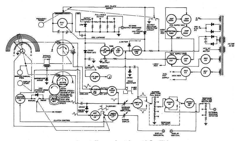
Figure 2-1. Elementary schematic diagram of the Type 1025-A Standard Sweep-Frequency Generator.
