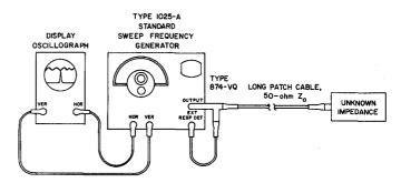
Figure 4-1. Measurement set-up for display of VSWR.
