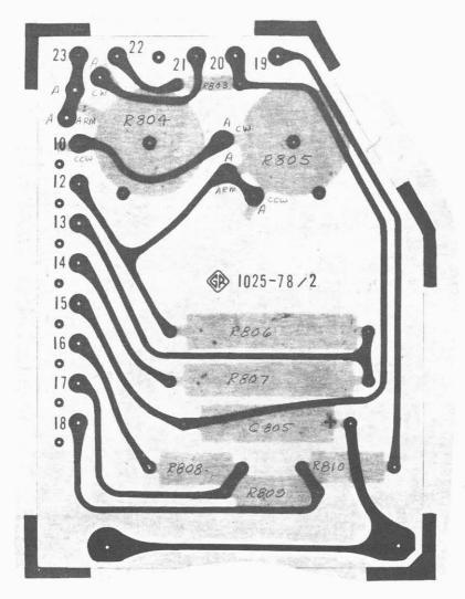
Figure 6-11. Etched-board layout for power supply (A8) in the Type 1025-A.
