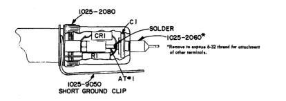
1800-2600 ALTERNATE LONG GROUND-CLIP ASSEMBLY -1800-8570 CDC-1010 This assembly can replace the Type 1025-9050 Short Ground Clip for use below 50 Mc.
