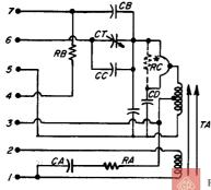
Figure 6-12. Schematic diagram of frequency-turret sectors for the following ranges:
