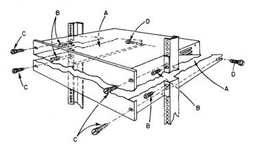
Figure 3-1. Installation of relay-rack model, Type 1025-AR.
