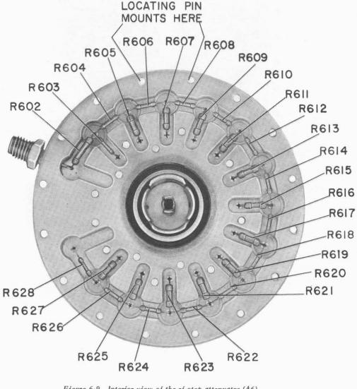
Figure 6-9. Interior view of the rf step attenuator (A6) of the Type 1025-A. File Courtesy of GRWiki.org
