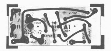
Figure 6-5. Etcbed-board layout for metering circuit (A1) of the Type 1025-A.
