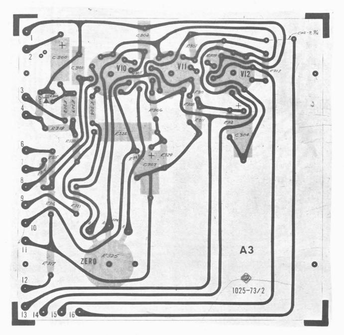
Figure 6-6. Etched-board layout for -150-volt regulator and meter circuit (A3) of the Type 1025-A
