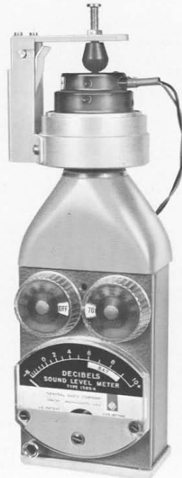
Figure 4. Type 1560-P82 Earphone Coupler used on Type 1565-A Sound-Level Meter.
