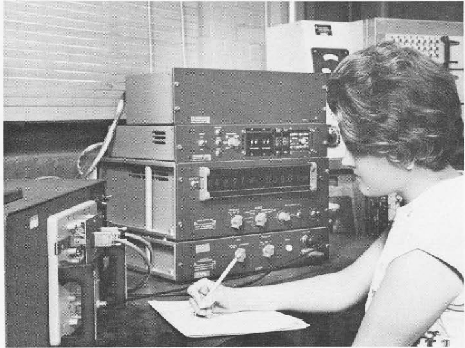
Figure 6. Bridge-scanner system used in environmental tests on dipped-mica capacitors.
