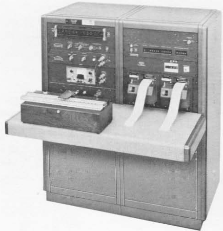
Figure 4. An automatic capacitor-test system produced by General Radio.
