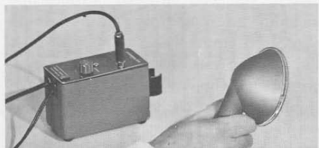
Lamp, at end of five-foot cable, can be held in hand as shown here or attached to case as shown on page 9.
