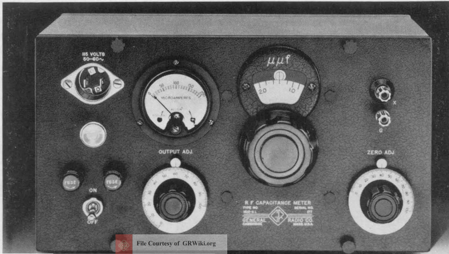
Figure 1. Panel view of the Type 1612-AL R-F Capacitance Meter, showing open capacitance scale at low end of range.
