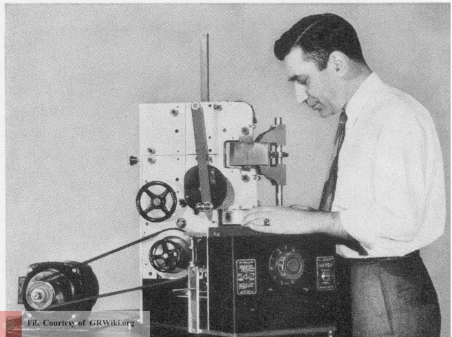
Figure 1. New Type 1700-B Variac Speed Control installed on toroidal winding machine.
