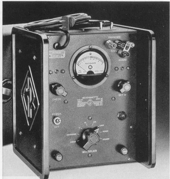
Figure 1. View of the megohmmeter with cover removed to show panel.
