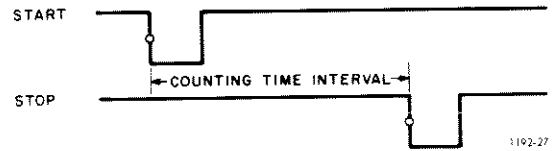
Figure 3-4 Time-interval measurement start and stop pulses.
