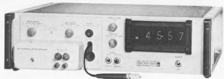
Figure 9. The 1820-P3 Dc Differential Adaptor, shown in place on the 1820-P2.
