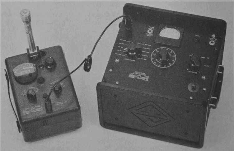
Figure 1a. Type 1550-A Octave-Band Noise Analyzer and Type 1551 Sound-Level Meter interconnected for analysis for airborne sound.
