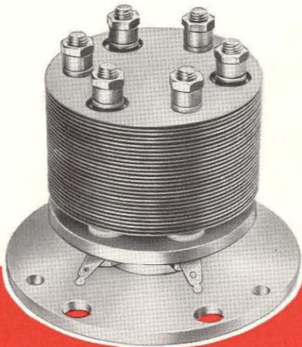
Figure 1. View of the 1000-pf capacitor removed from its cabinet and sealed container, showing the construction of the plate stack.
