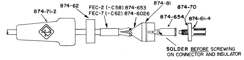
Slide outer transition piece (874-653) up to insulating bead (874-70), align keyways, and arrange braid over small end. Cover with cable ferrule and crimp in place. Crimping can be easily accomplished by holding ferrule against a sturdy surface and pinching and pushing simultaneously with a pair of ordinary gas pliers as illustrated.\*
