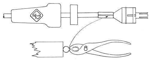
Slip outer conductor (874-60-3) over bead (874-70) and outer transition piece so that keys engage keyways.
