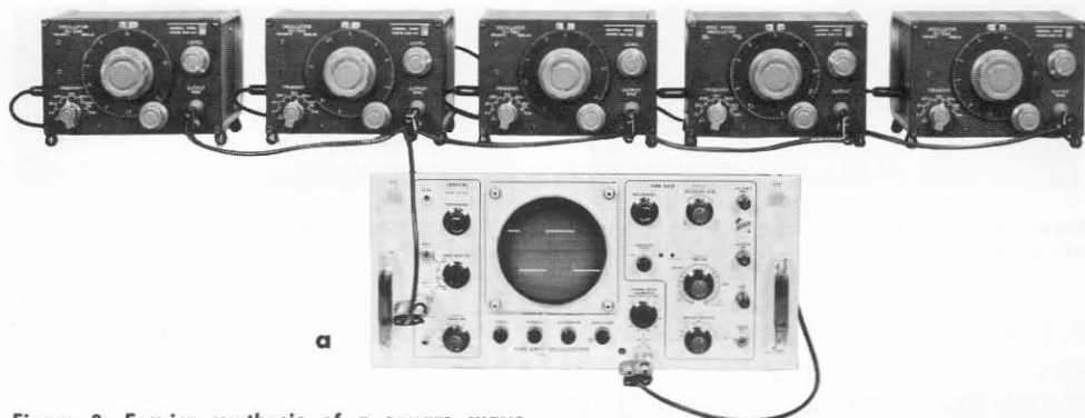
Figure 8. Fourier synthesis of a square wave. (a) Five oscillators synchronized to the first five odd-order harmonics of a square wave. The sinusoidal outputs of the oscillators are adjusted for phase coherence and summed in the ratio of their respective Fourier coefficients to make a Fourier approximation to the original square wave. (b) The original synchronizing square wave. (c) The coherent fifth harmonic. (d) The synthesized square wave.
