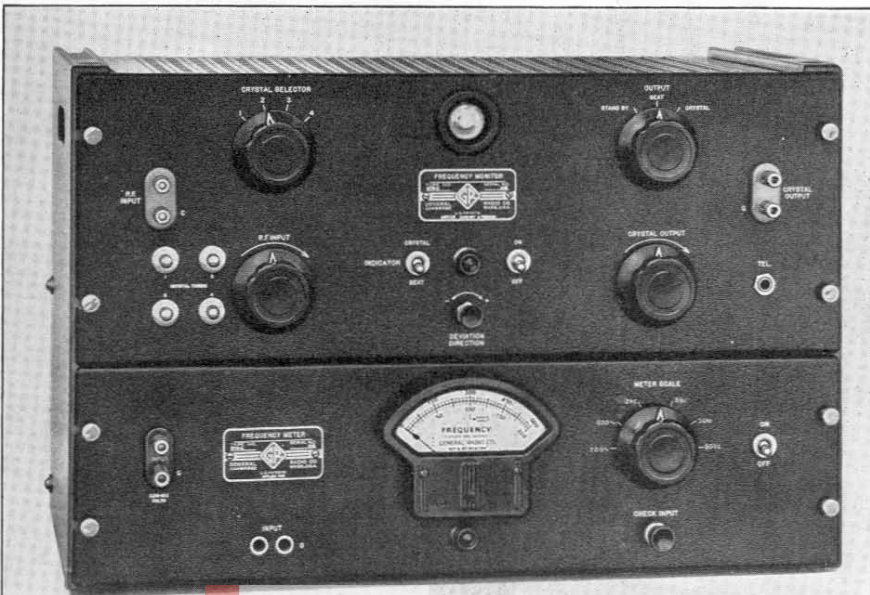
Figure 1. View of the TYPE 1175-A Frequency Monitor with TYPE 1176-A Frequency Meter.
