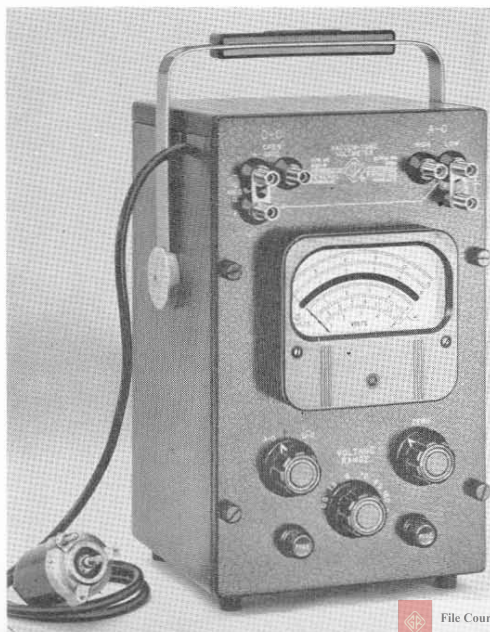
Figure 1. View of the Type 1800-B Vacuum-Tube Voltmeter. It is similar in appearance to its predecessor, the Type 1800-A, but includes a panel switch for d-c polarity selection.
