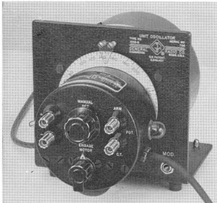
(Above) View of Type 907-R-144 X-Y Dial Drive, installed on a u-h-f Unit Oscillator.
