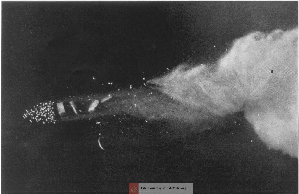
FIGURE 3. A Microflash photograph of the explosion of a shotgun shell as it leaves the muzzle of the gun, which is out of the picture at the left. Note that the wads can be seen as well as the cluster of shot.
