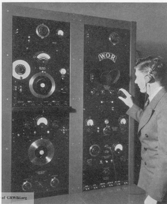
FIGURE 2. Equipment for measuring modulation and distortion consists of wave analyzer, beat-frequency oscillator, modulation meter, distortion and noise meter, range-extension filter, and cathode-ray oscillograph. These are conveniently mounted on a pair of relay racks as shown here.
