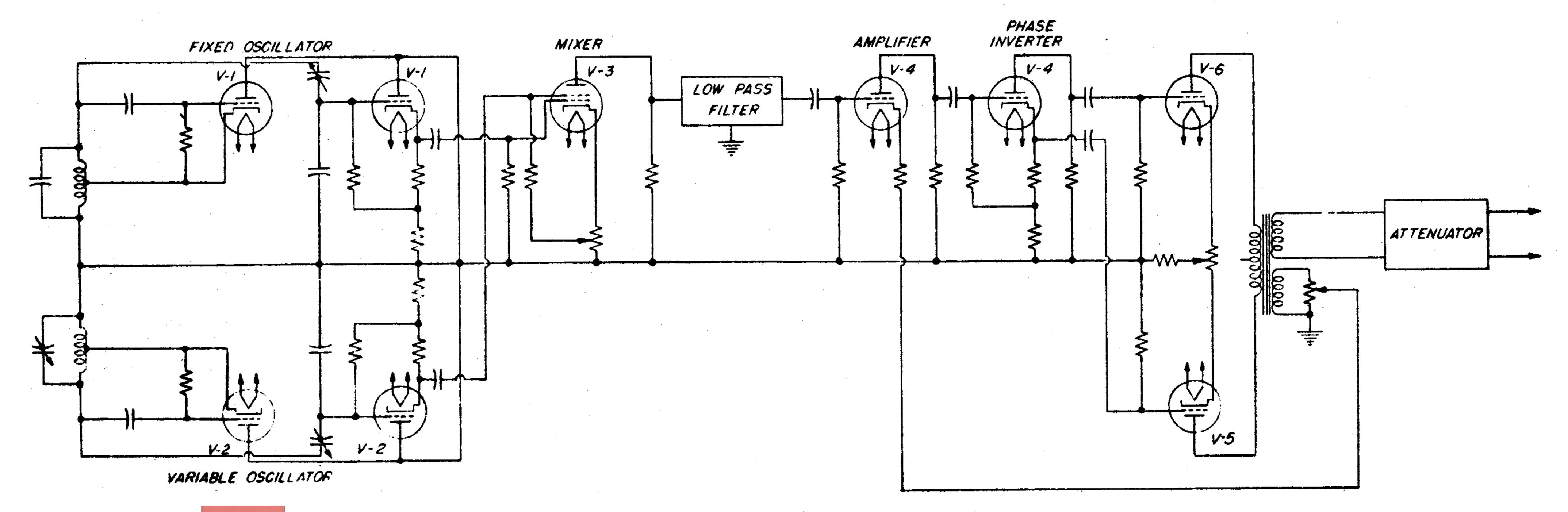
Figure 1. Schematic Diggrame Courtesy of GRWiki.orgBeat-Frequency Oscillator.
