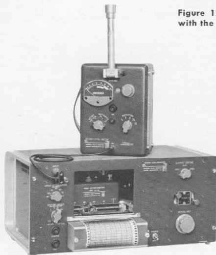
Figure 13. View of the Graphic Level Recorder bench-mounted with the Type 1151-AP Digital Time and Frequency Meter and the Type 1136-A Digital-to-Analog Converter.
