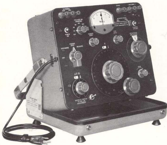
Figure 1. Panel view of the Type 1644-A Megohm Bridge. The Flip-Tilt case permits the panel to be positioned at any desired angle. Inset shows the older Type 544-B.
