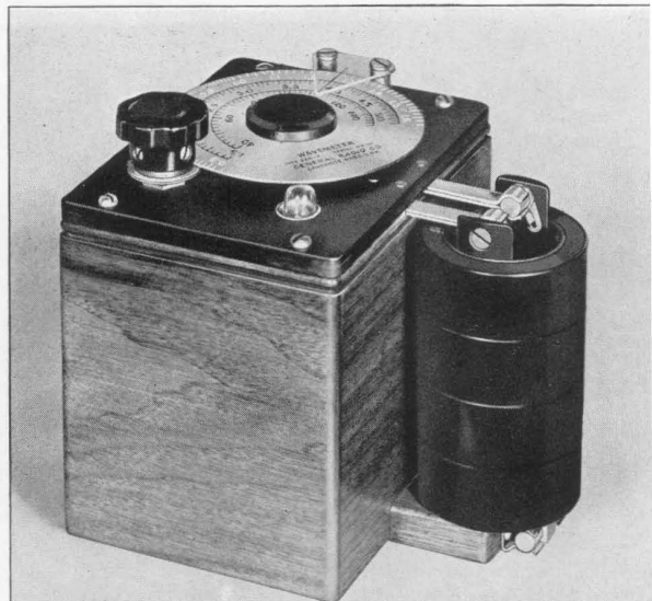
FIGURE 1. View of the TYPE 566-A Wavemeter showing how coils are stored when not in use.
